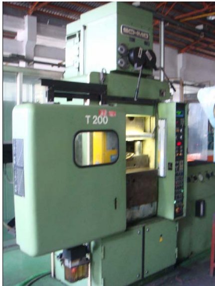
Fig. 4. T 200 cold rotary forging press.
